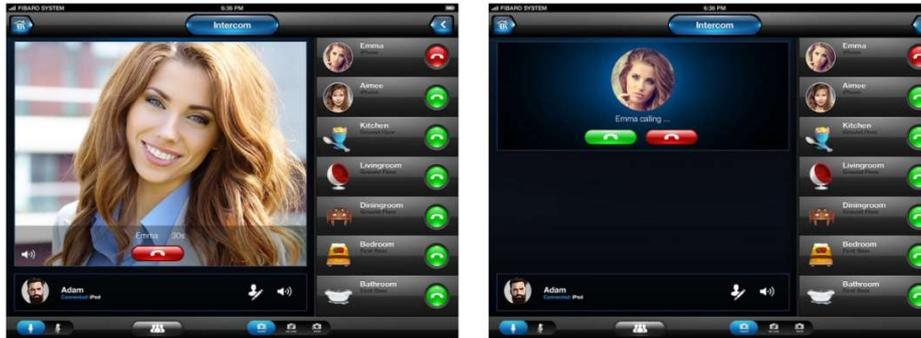
6. Access the **FIBARO Intercom App** on your smartphone/tablet and set up your details. Press **Overwrite** on the first screen to remove the need to enter your credentials again for the Fibaro HC2. Allow Microphone, Camera, Notifications and Contacts access for 'Fibaro Intercom' App. You will be asked to create and name a new **VoIP client** specific to the smartphone/tablet used during this registration step. This is the device that will be called when the intercom's dial button is pressed.
