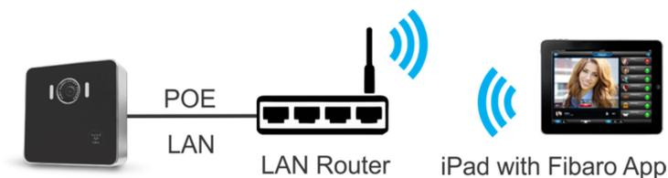
2. Connect the VBell™ Video VoIP Intercom to your router using a CAT6 ethernet cable (not included) and to a power supply if your router does not support POE (Power over Ethernet). Power will be provided to the device via the ethernet cable and the Intercom's LED will start flashing. Wait until the Intercom completes the start-up process, it usually takes less than one minute. The Intercom is set to use the DHCP boot protocol by default
