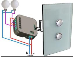
Example of wiring with Clipsal Saturn range 2 gang wall plate and two 30/60PBBPL Bell Press Mechanism.
