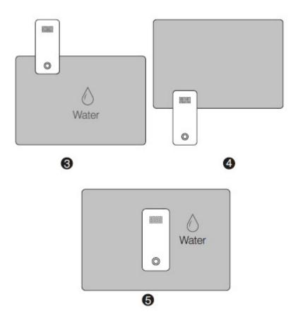
These situations will cause Water Sensor 6 to send a water presence or trigger event to your gateway. Should water clear from the area where Water Sensor 6 is installed, the sensor will also send a separate command to your Z-Wave gateway informing it that there is no more water in the area.
