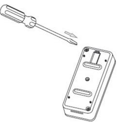
After securing the sensor plate your Water Sensor unit will have the waterproof rating of IP65.
