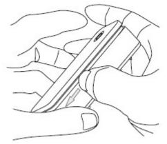
3. Once the battery cover is separated from the Sensor Unit, you can pull out and change the battery located in the center of the Water Sensor 6 hardware.
