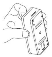
b. Push or move your fingernail along the gap between the battery cover and Sensor unit.
