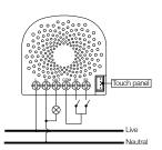
Wiring diagram of 2-Wire system.
