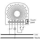
Note: The "N" terminal should be connected to the "L" terminal when the Nano Dimmer is installed by 2-Wire system.
