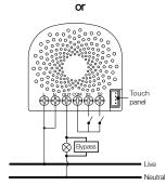
All above wiring diagrams show that the Nano Dimmer uses 2-Way or momentary button switches as the external manual switch.
